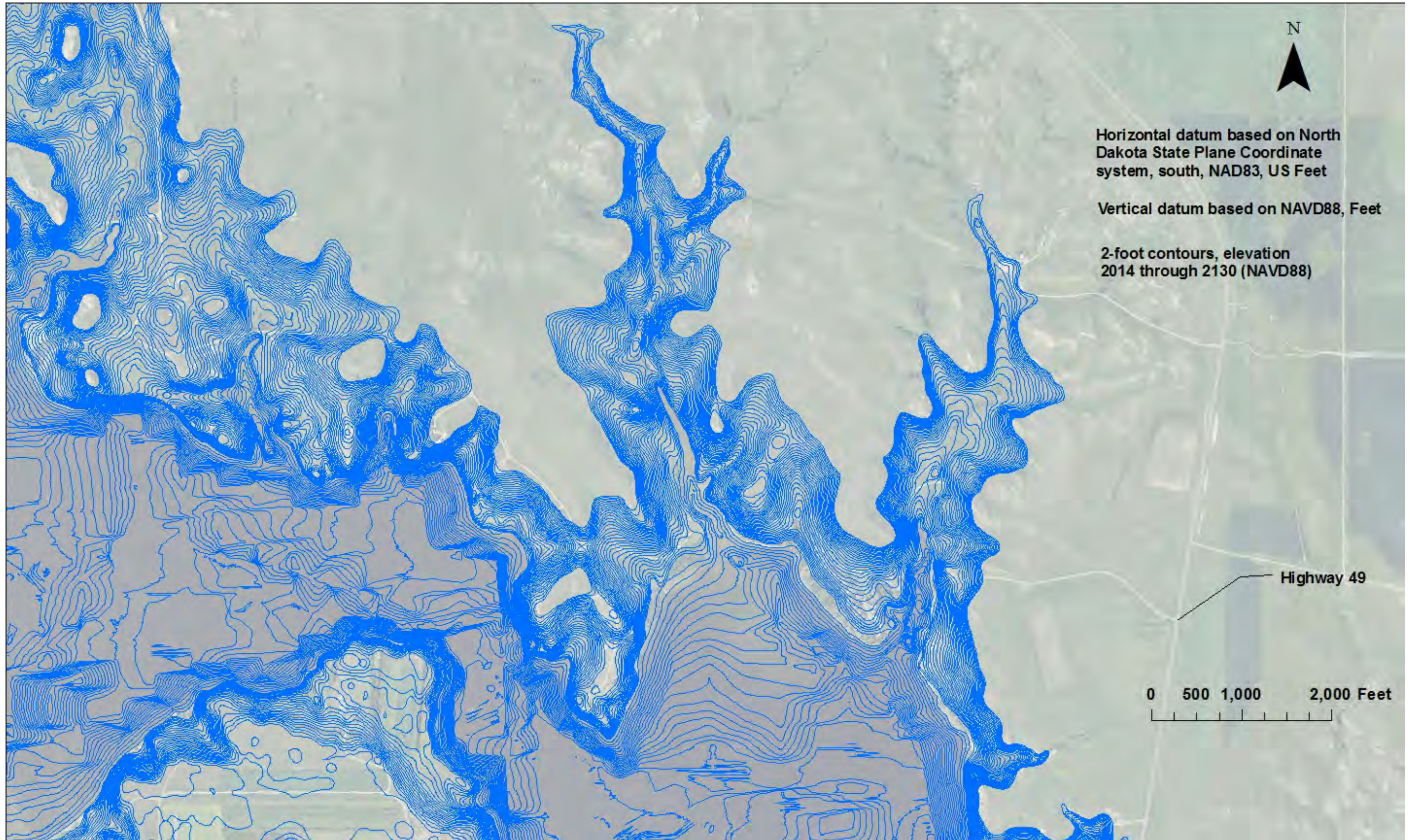
Figure 13 - Lake Tschida developed 2-foot contours from 2013 bathymetric survey and imported data coverages, 2 of 16 (NAVD88/GEOID12A).
