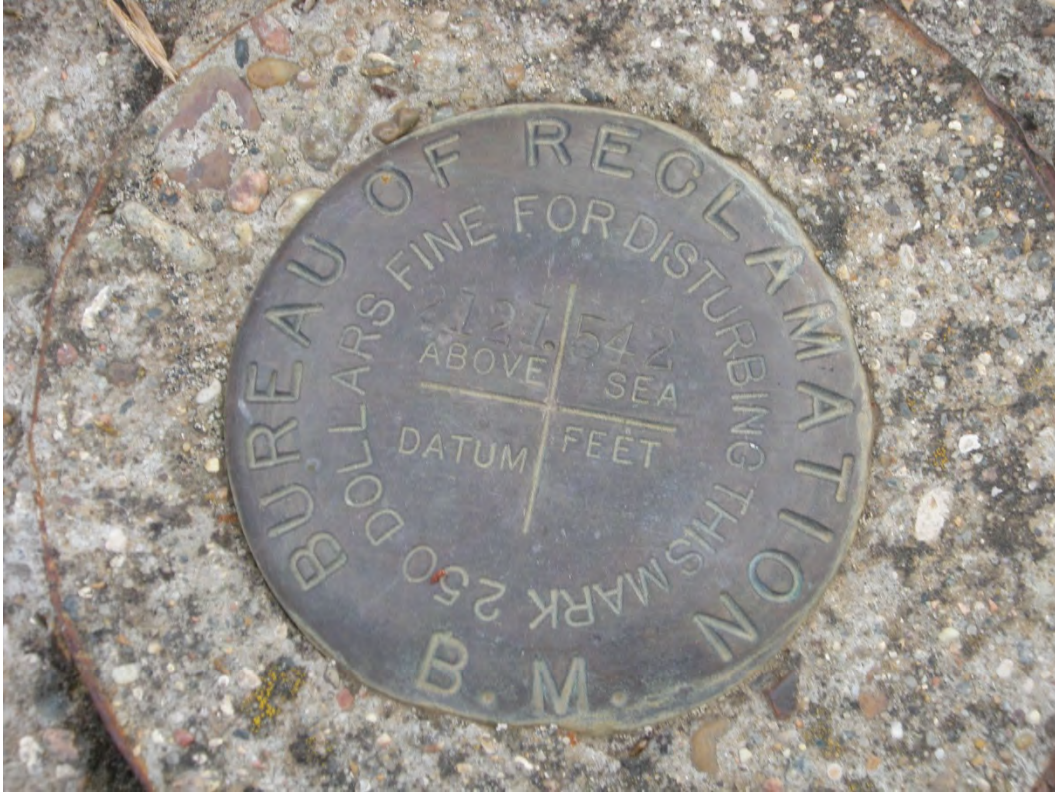
Figure 4 - Bureau of Reclamation stamped "2121.542."
