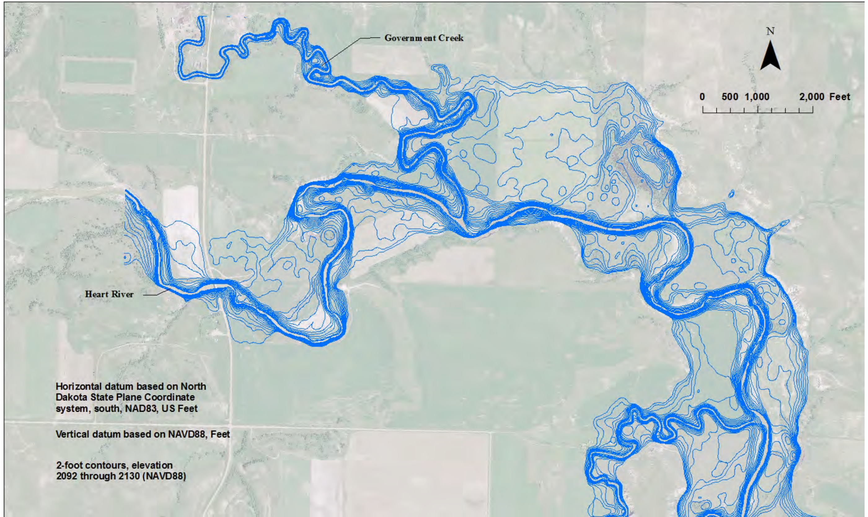
Figure 27 - Lake Tschida developed 2-foot contours from 2013 bathymetric survey and imported data coverages, 16 of 16 (NAVD88/GEOID12A).
