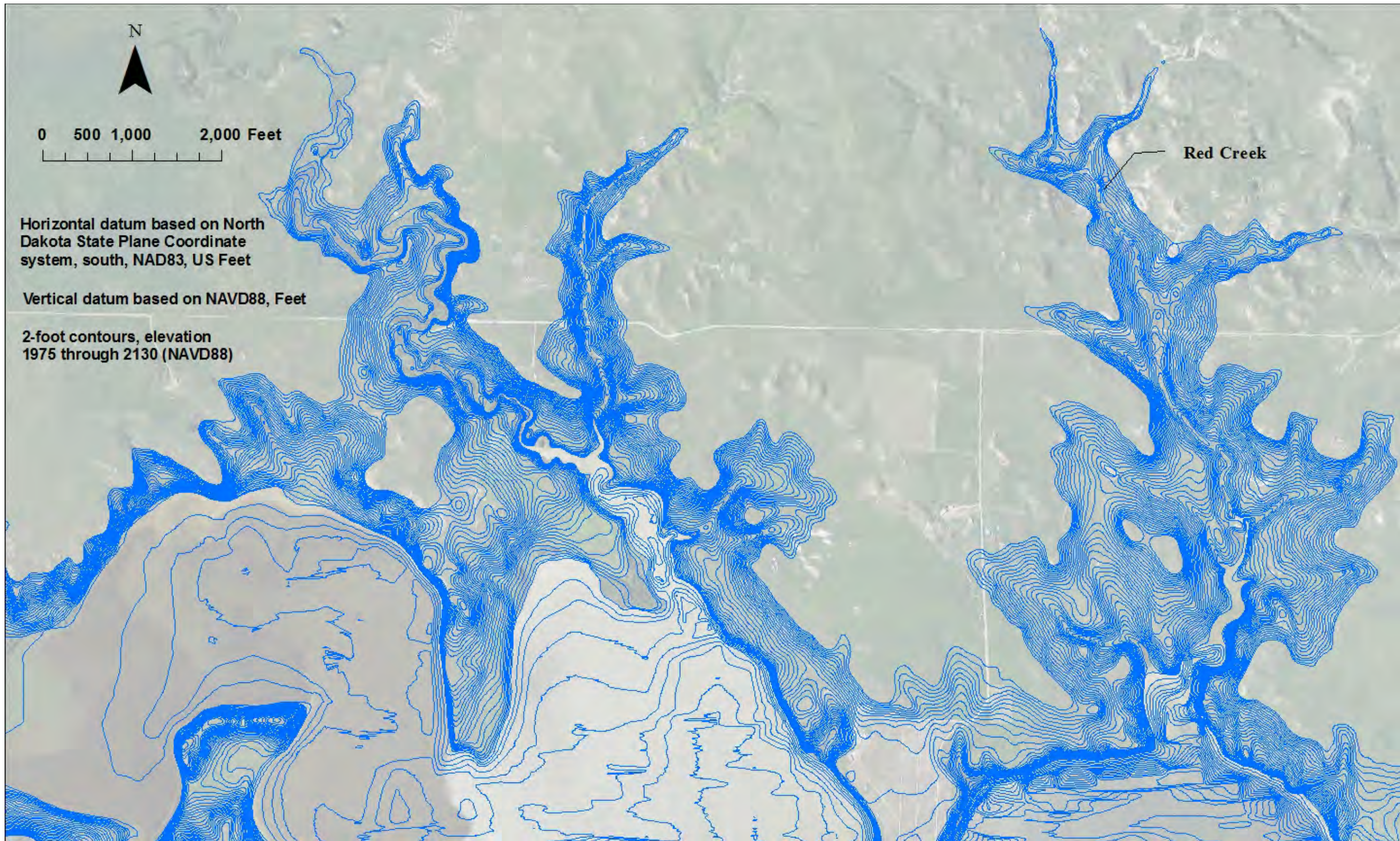
Figure 18 - Lake Tschida developed 2-foot contours from 2013 bathymetric survey and imported data coverages, 7 of 16 (NAVD88/GEOID12A).
