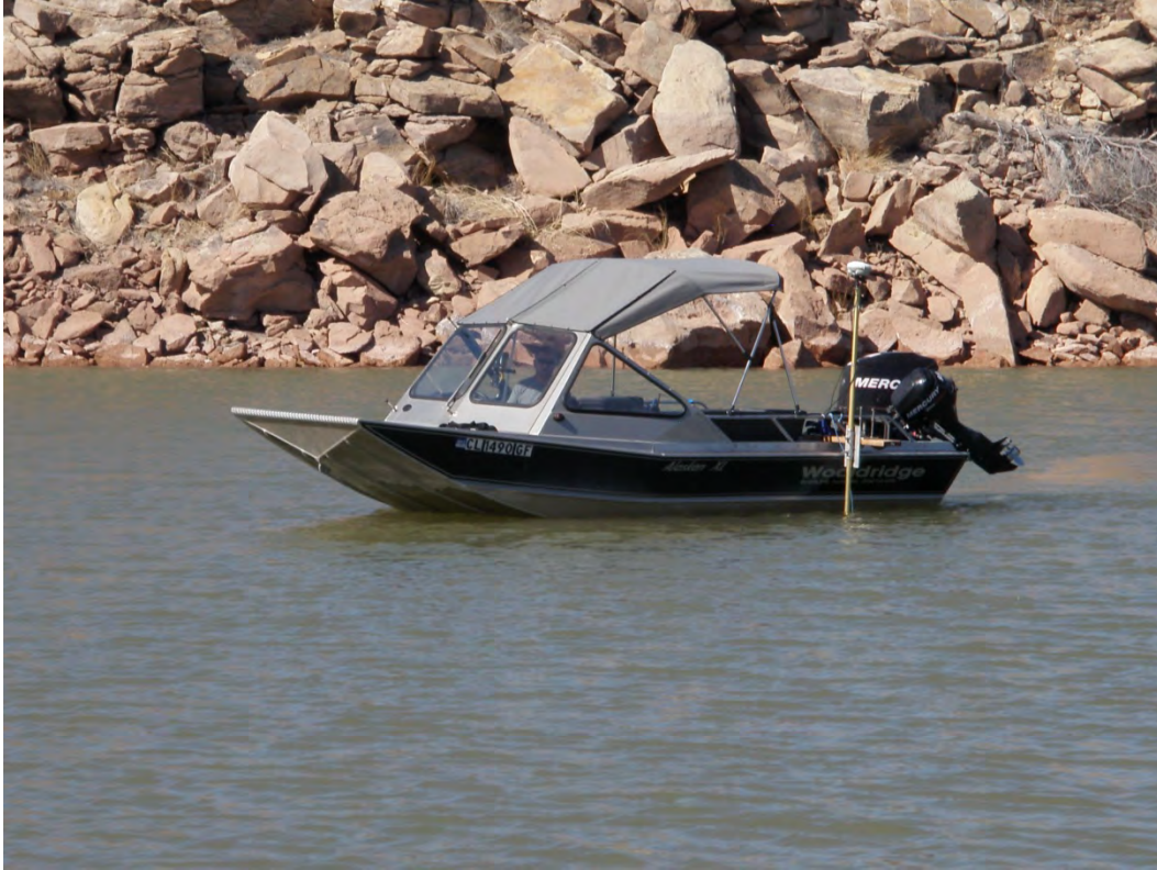
Figure 6 - Survey vessel for reservoir mapping with mounted transducer on side (Lake Sumner-New Mexico, March 2013)
