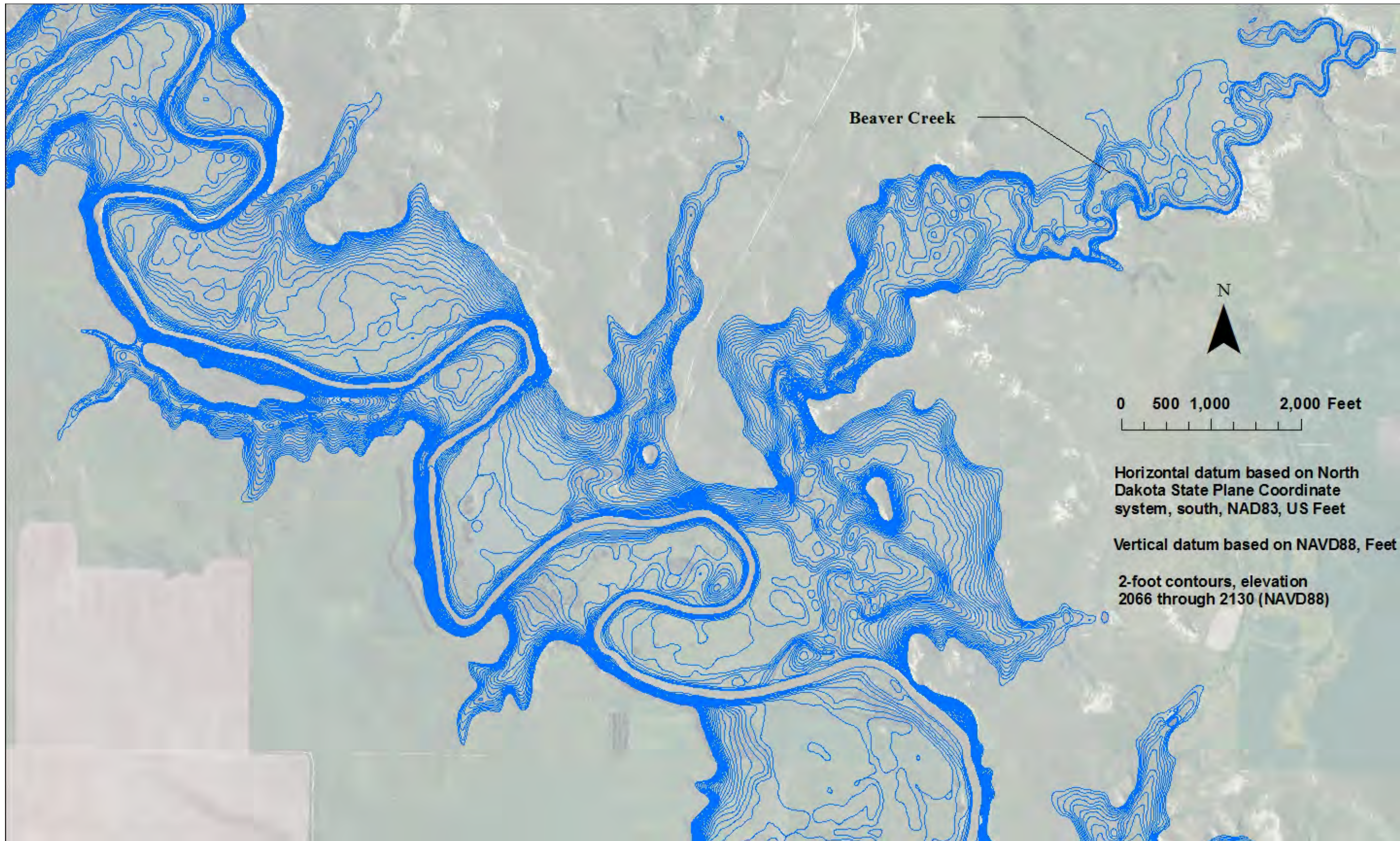
Figure 23 - Lake Tschida developed 2-foot contours from 2013 bathymetric survey and imported data coverages, 12 of 16 (NAVD88/GEOID12A).
