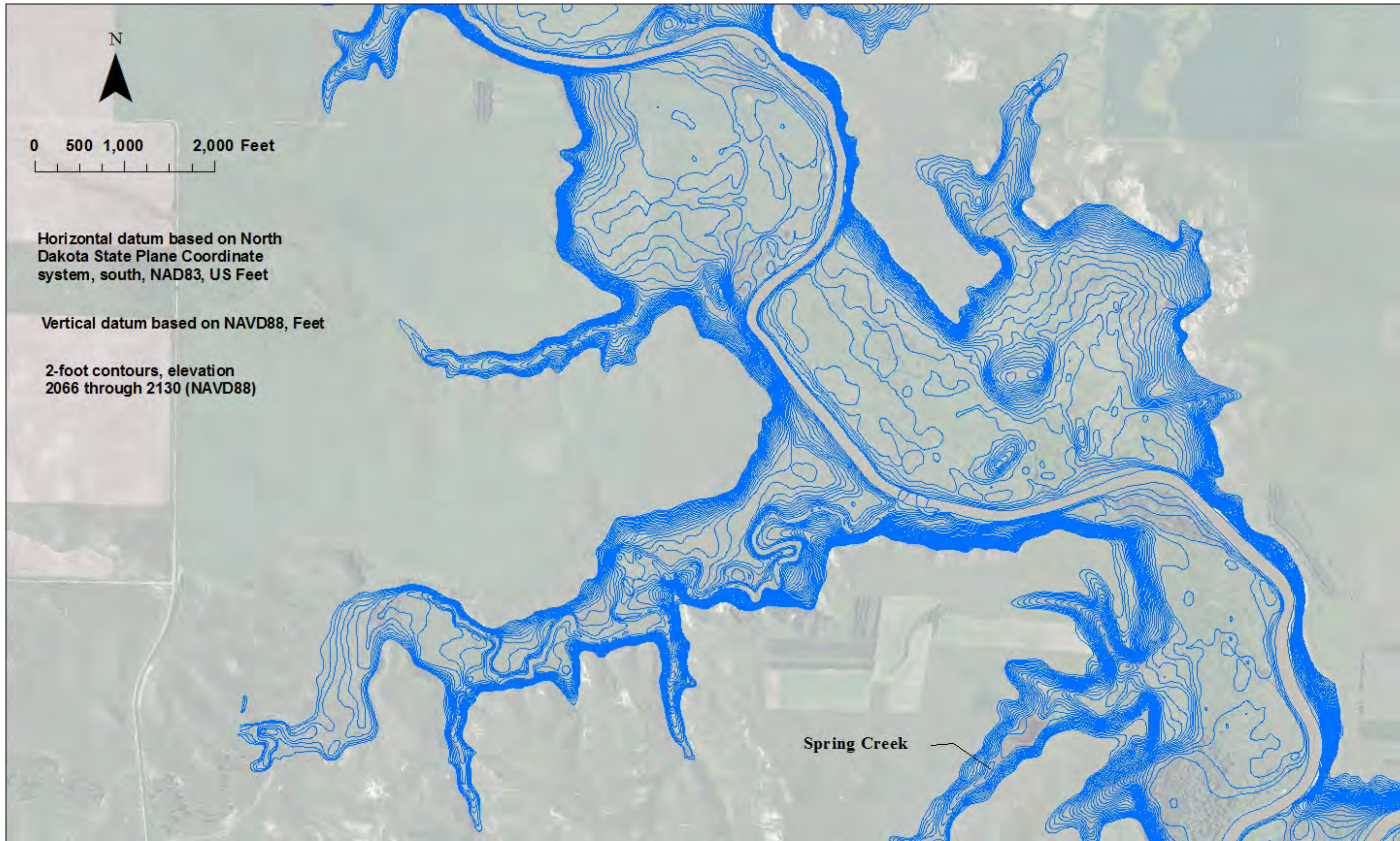
Figure 22 - Lake Tschida developed 2-foot contours from 2013 bathymetric survey and imported data coverages, 11 of 16 (NAVD88/GEOID12A).
